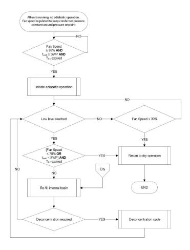
SWP: ambient temperature switch point Tamb: ambiant dry bulb temperature Tpc: pre-cooler timer to avoid hunting in adiabatic activation/deactivation (default 5 min - adjustable)
