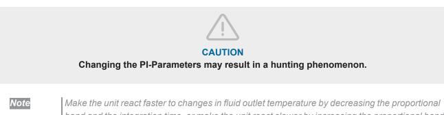
Make the unit react faster to changes in fluid outlet temperature by decreasing the proportional band and the integration time, or make the unit react slower by increasing the proportional band and integration time.
