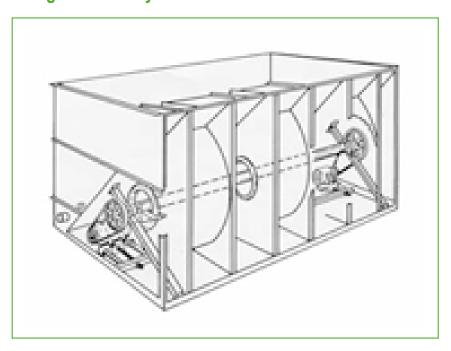
The installation of a Baltiguard  $^{\tiny{\scriptsize{\scriptsize{\scriptsize{B}}}}}$  drive system
