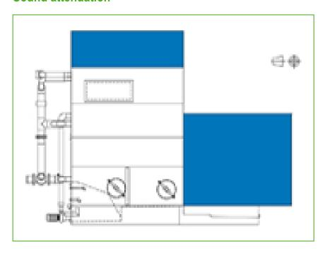
HFL cooling towers use **quiet centrifugal fans**, **but to reduce noise even further**, **you can** extend your HFL cooling tower with sound attenuators at the air intake and discharge points.
