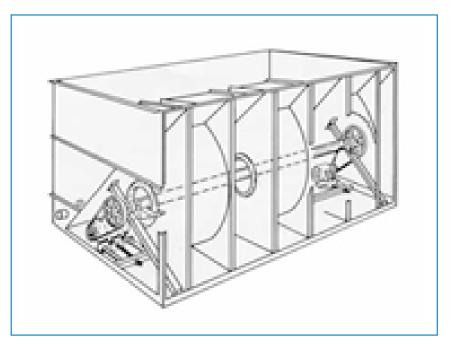
The installation of a Baltiguard<sup>®</sup> Drive System
